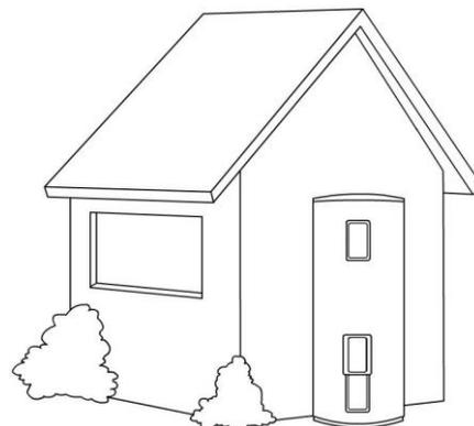
The water heater is to be installed at ground or floor level and must stand vertically upright on a stable base as acceptable to local authorities. The base of the water heater is made of corrosion resistant material, and it may be placed directly in contact with the supporting surface. It is not necessary to allow for free air circulation under the base of the water heater.
